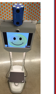
Figure 8. Our social robot platform: A Beam (Suitable Technologies, Inc.), equipped with the Occam Omni Stereo rgbd camera (Occam Vision Group).
