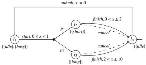
Figure 1: An example APTA specification for a scheduler component.
